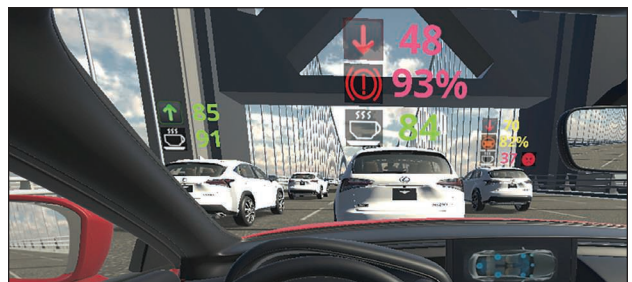
FIGURE 7 An example illustration of a meta-empowered ADAS. Information is displayed on the ego vehicle's windshield as the AR-based HUD, which includes neighboring drivers' 1) proficiency scores and their trends, 2) possibilities of certain potential actions (e.g., hard braking and lane change), and 3) current mood score.
